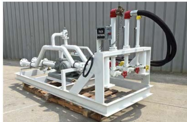
Control Manifold with EPA Compliant Flow Monitoring
